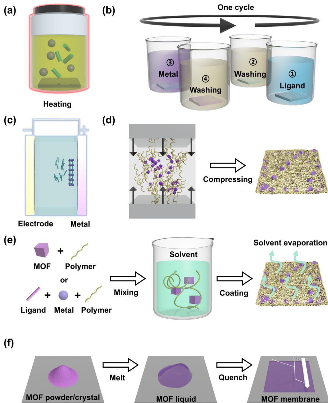
**Fig. 3.** Fabrication methods of proton-conducting MOF membranes. (a) Solvothermal/hydrothermal method; (b) dip coating method; (c) anodic deposition method; (d) compression molding method; (e) solution evaporating casting method; (f) melt-quenching method.
