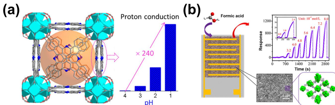
**Fig. 8.** Representative MOF-based proton sensors. (a) The pH responsiveness of zirconium-based MOFs; reprinted with permission from Ref. [35], Copyright © 2021, American Chemical Society. (b) Efficient formic acid detection using MOF-802 membrane device; reprinted with permission from Ref. [36], Copyright © 2021, American Chemical Society.
