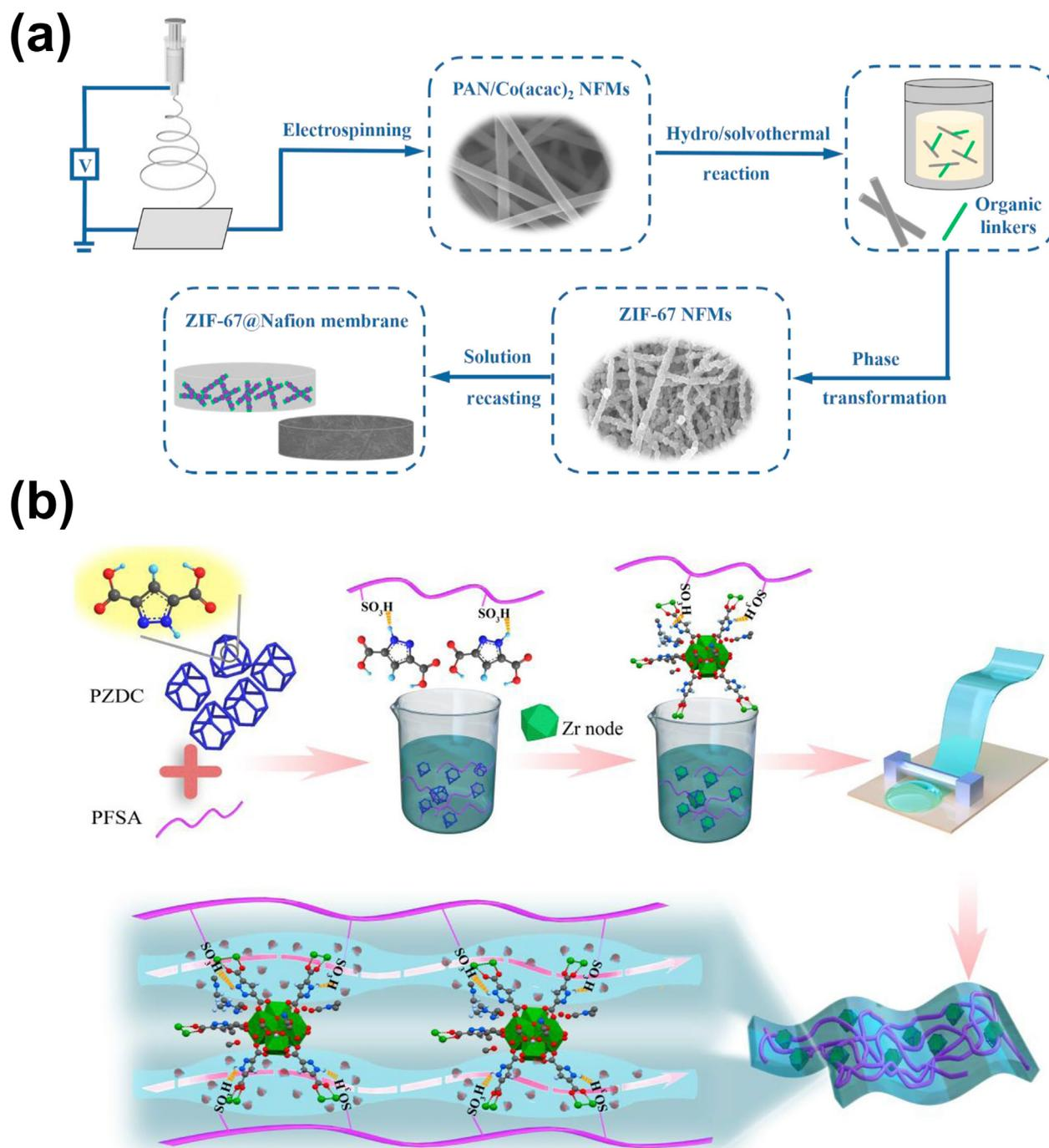
**Fig. 7.** Fabrication routes of ZIF-67 and NH-Zr MOF-based MMMs. (a) Fabrication routes of ZIF-67 NFMs and ZIF-67@Nafion composite membranes; reprinted with permission from Ref. [89], Copyright © 2021, Elsevier B.V. (b) Schematic illustration of NH-Zr MOF hybrid membrane preparation; reprinted with permission from Ref. [90], Copyright © 2023, Springer Nature.
