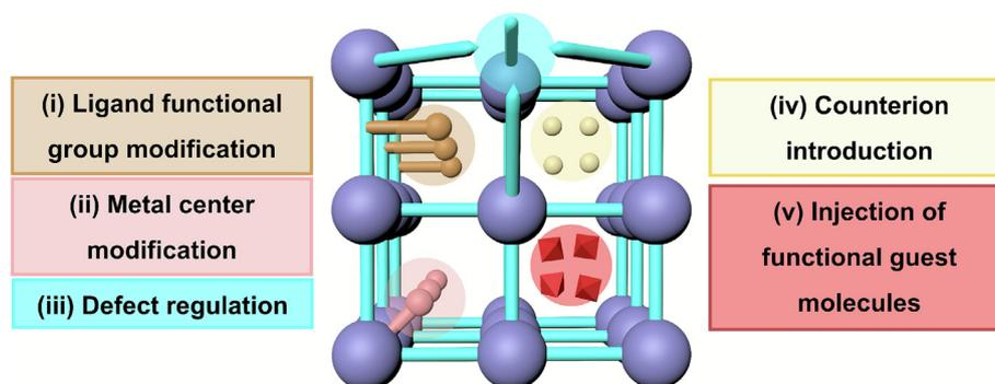
Fig. 2. Schematic illustration of design strategies for proton-conducting MOFs.
